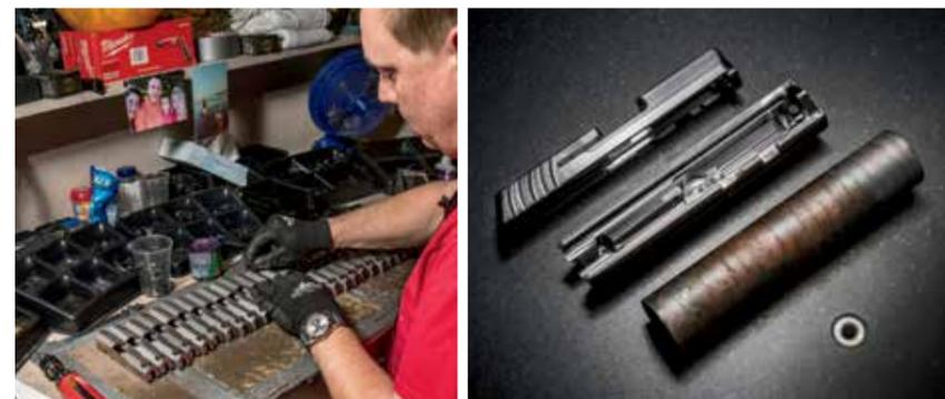
Every slide starts out as a section of round bar stock. After two machining steps, it's a slide.
