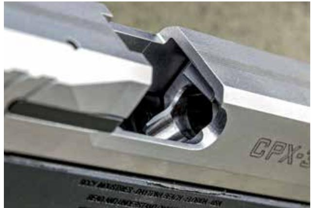
The adequately sloped feed ramp into the barrel aids in reliable operation with all types of .380-bullet profiles.
